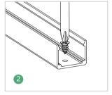
2.Adjust the aluminum profiles to the desired position, use a screwdriver to tighten the screws.
