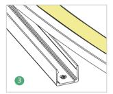
3.With the luminous surface facing up, fit the product into the aluminum profiles. Finished.
