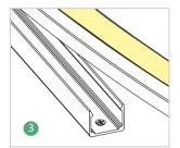
With the luminous surface facing up, fit the product into the aluminum profiles. Finished.
