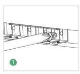
Fix the stainless steel flexible mounting profile into the pre-cut groove, use a screwdriver to tighten the screws.
