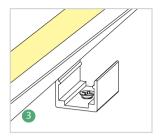
With the luminous surface facing up, firmly insert the product into the clips.
