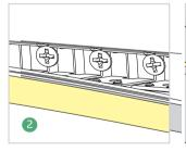
Embed the strip light into the groove, with the luminous surface facing outward.
