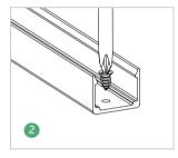
Adjust the aluminum profiles to the desired position, use a screwdriver to tighten the screws.
